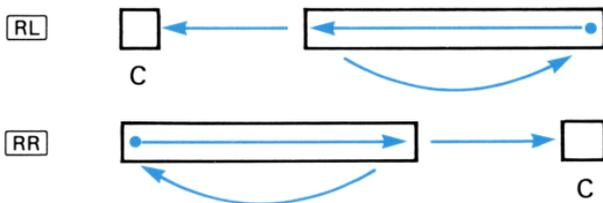
**Rotation Through the Carry Bit.** The `RLC` and `RRC` (*rotate left through carry* and *rotate right through carry*) functions respectively load the leftmost or rightmost bit of a word into the carry bit, and move the carry bit into the other end of the word.
