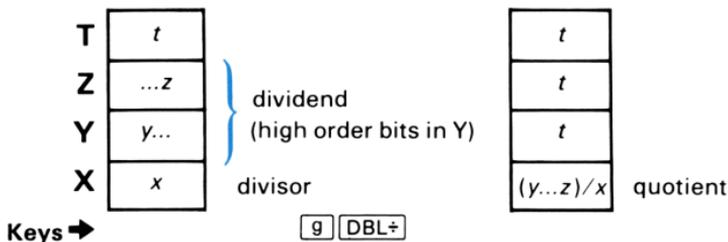
**Example:** The calculation of  $(-88 \div 11)$  in binary with word size 5 and 2's Complement mode is shown below.
