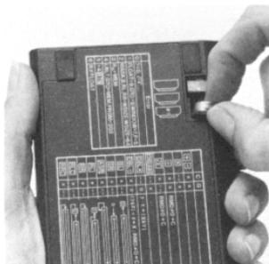
6. Insert the tab of the battery compartment door into the slot in the calculator case.
