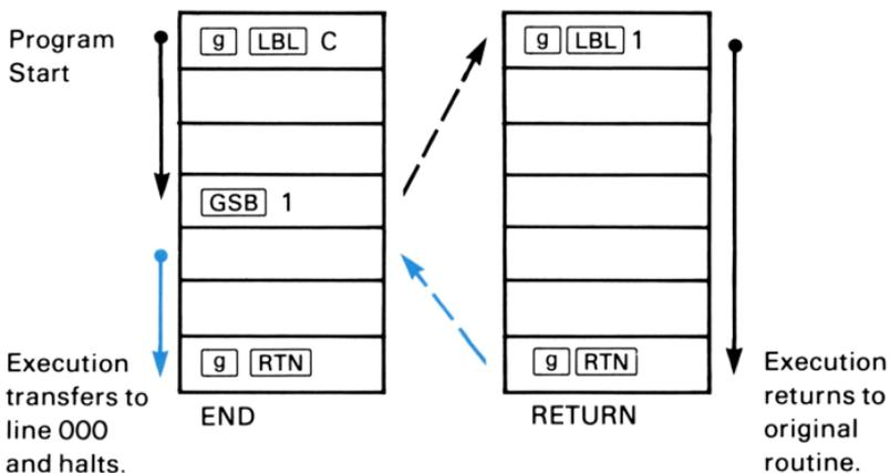
**Nesting.** Subroutine “nesting”—the execution of a subroutine within a subroutine—is limited to a nest of subroutine returns four levels deep (not counting the main program level).
