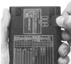
**Note:** In the next two steps, be careful not to press any keys while batteries are not in the calculator. If you do so, the contents of Continuous Memory may be lost and keyboard control may be lost (that is, it will not respond to keystrokes).
