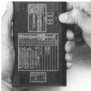
3. Grasp the outer edge of the battery compartment door, then tilt it up and out of the calculator.
