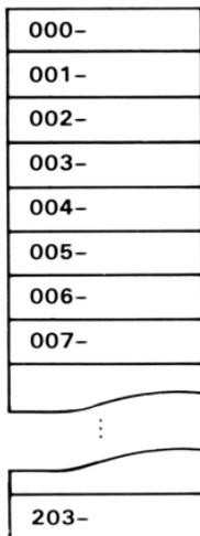
There are 203 bytes (lines) of total memory for programming and storage. All memory is initially in storage registers and is automatically allocated to program memory as necessary.
