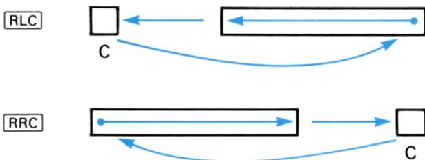
**Rotating More Than One Bit at a Time.** Given a bit pattern in the Y-register and  $n$  in the X-register, pressing `f RLn`, `f RRn`, `g RLCn`, or `g RRCn` will rotate the pattern  $|n|$  bits. The stack drops, placing the result in the X-register.
