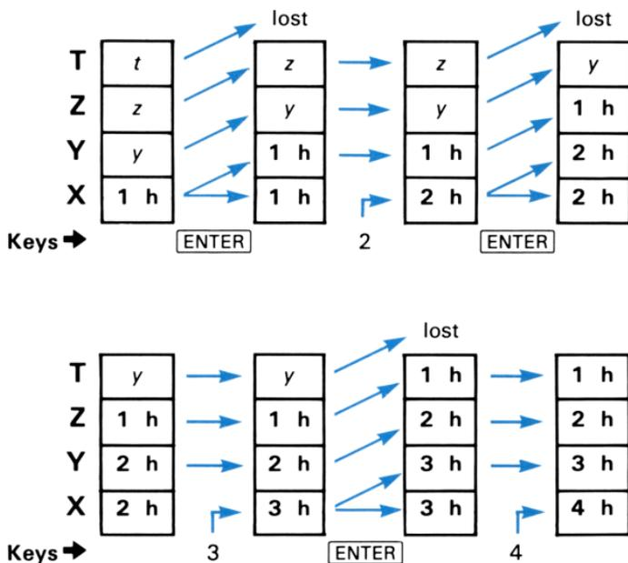
In addition to **ENTER**, there are three other functions that rearrange the stack:
