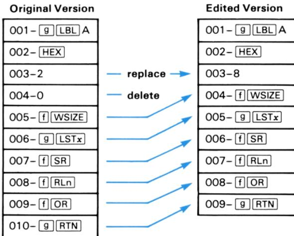
Making a deletion or addition of a program line alters the line numbers of those program lines following. By editing the program from the end backwards, you can preserve the original line numbers of parts of the program not yet edited. This allows you to access remaining lines by their original numbers. The editing steps below assume the concatenation program occupies line 001 to 010.
