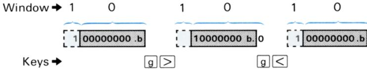
**Example:** The following scrolling and `WINDOW` functions can be used to view the entire X-register contents. The word size used is 16 bits.
