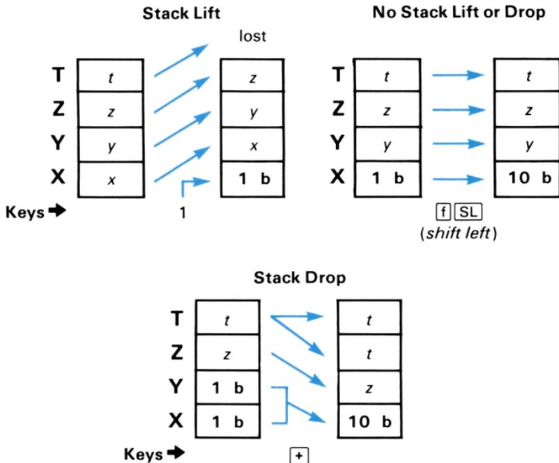
Typically, one-number functions (as defined in the previous section) result in no stack movement, while two-number functions *usually* result in a stack drop.
