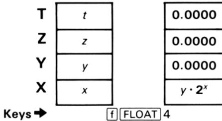
If  $y \cdot 2^x$  is greater than  $9.999999999 \times 10^{99}$ , flag 5 (out-of-range) is set and the overflow display (all 9's) results. If there is no overflow, flag 5 is cleared.
