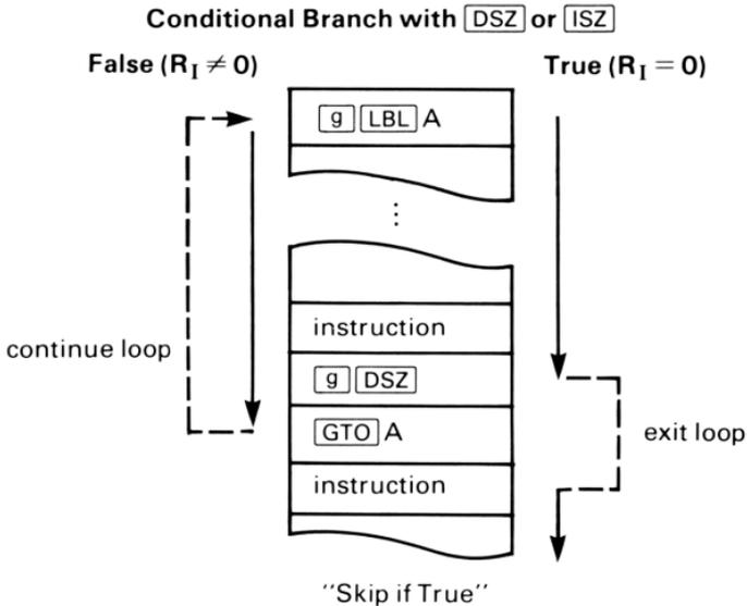
The value in  $R_1$  is interpreted according to the current complement mode. It can be positive or negative, in integer or floating-point format. The instructions `DSZ` and `ISZ` do not affect the status of the carry and out-of-range flags.
