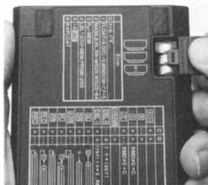
7. Lower the battery compartment door until it is flush with the case, then push the door inward until it is tightly shut.
